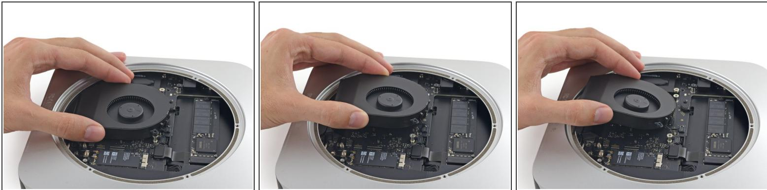
ⓘ The fan connector is trapped under the edge of the fan and cannot be disconnected until the fan is moved.
