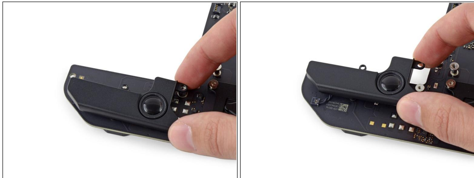
**⚠ Do not attempt to remove the speaker entirely as it is still attached to the logic board.**
