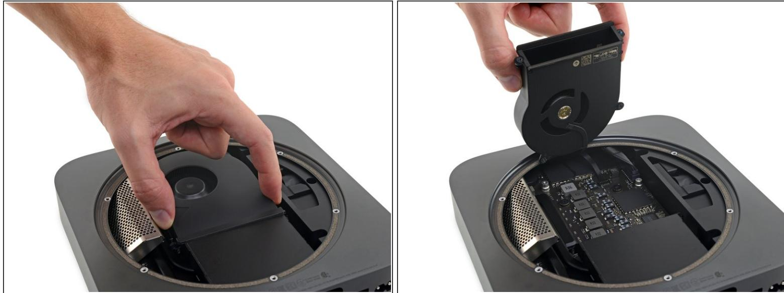
**⚠** Don't try to remove the fan completely in this step—just lift it so you can access the cable underneath.
