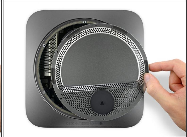
! Do not completely remove the antenna plate; it is still connected to the Mac mini by an antenna cable.
