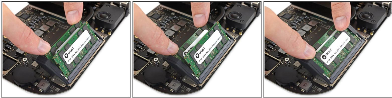
Finally, press the top edge of each RAM module to swing it down toward the logic board until the retaining clips on each side snap into place.
