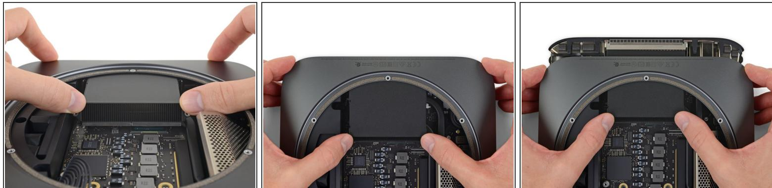
**⚠** In this step, you'll push the logic board free from the clips holding it to the frame. **Push only where directed** or you may damage the fragile cooling fins.
