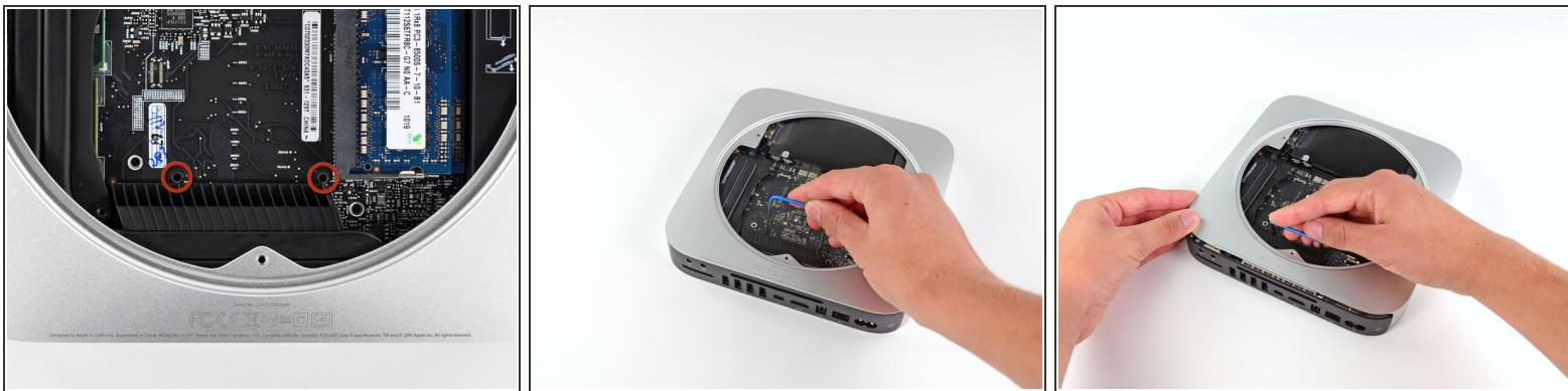
**⚠** To remove the logic board, two cylindrical rods must be inserted into the holes highlighted in red. Inserting instruments into any logic board holes other than the ones highlighted in red may destroy the logic board.
