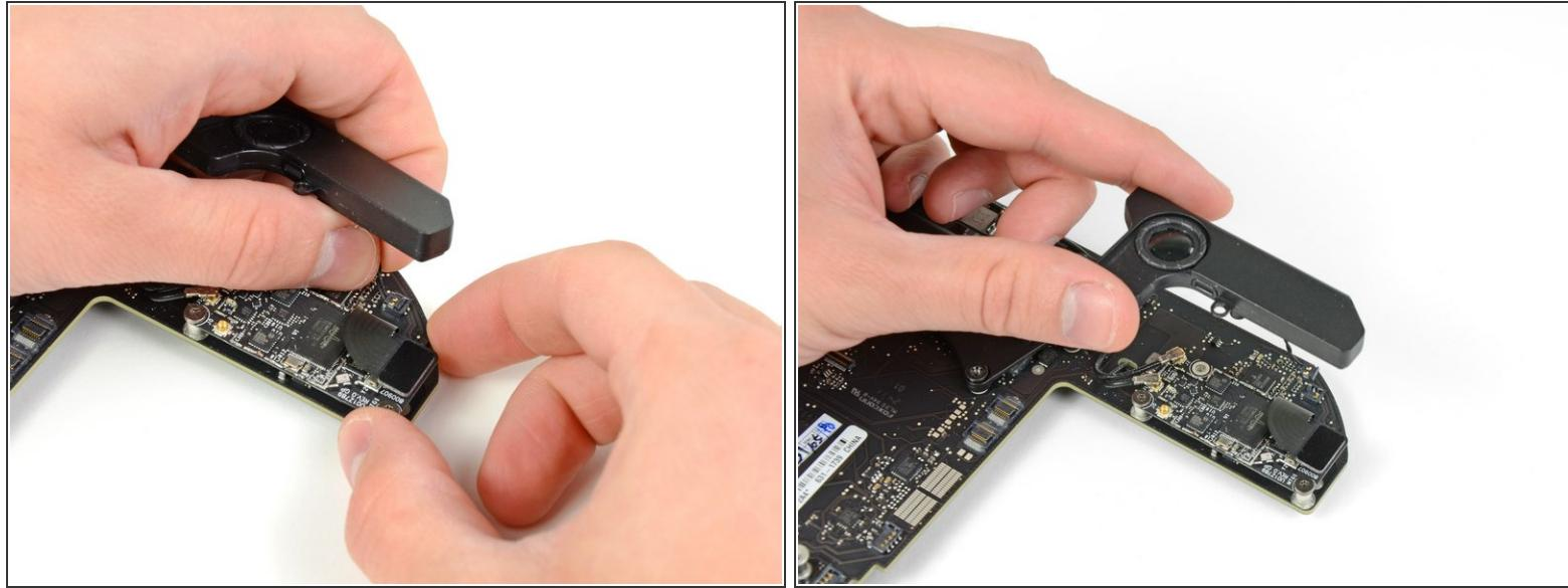
**⚠** Lift but do not remove the speaker assembly, as it still remains connected to the logic board via the speaker connector.
