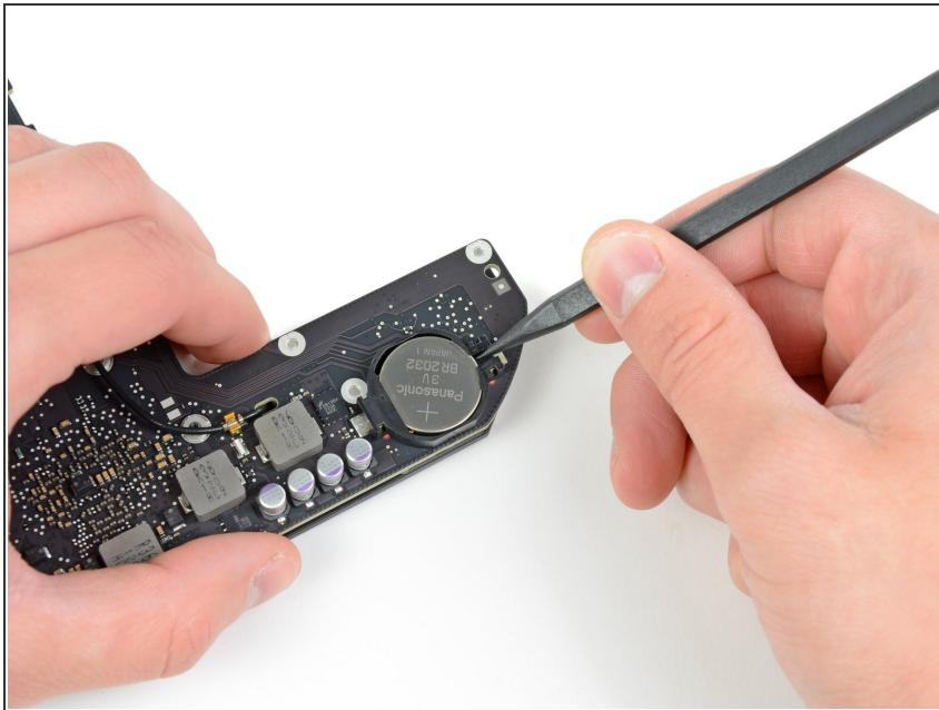
*i* The PRAM battery is located on the top side of the logic board.
