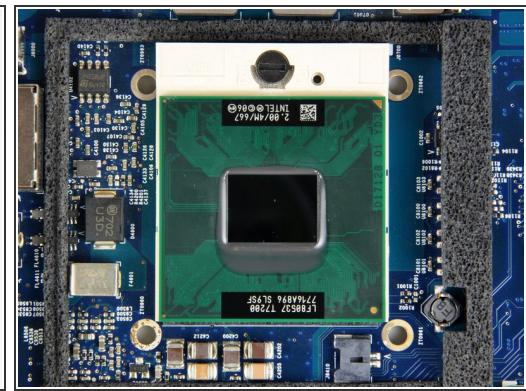
**⚠** Processors are extremely sensitive to electrostatic discharge. Only handle your processor by its edges.
