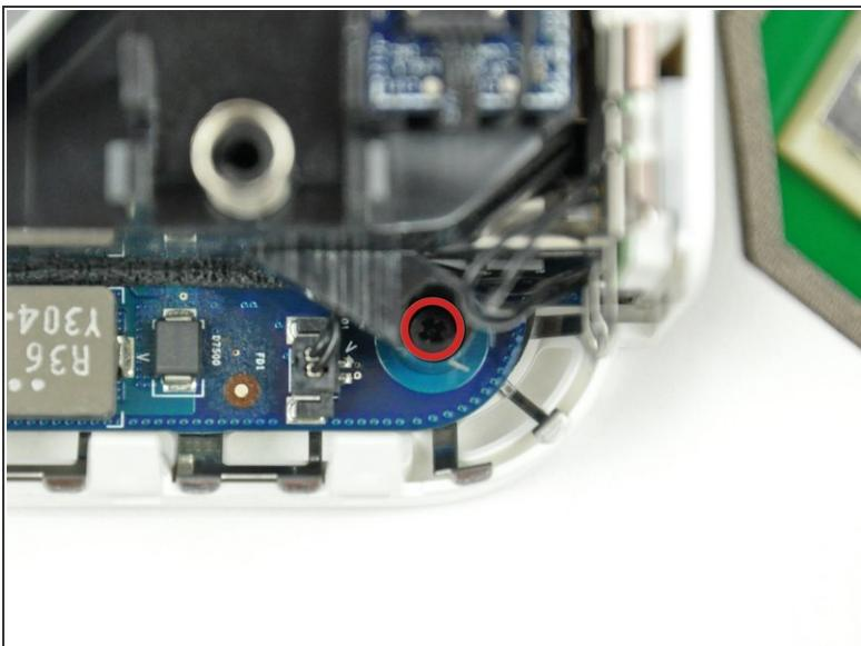
*(i)* In the next few steps, you will remove the four Phillips screws securing the internal frame to the bottom case. Included in each step is an overview picture showing the general location and a closeup showing the actual screw.
