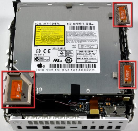
**⚠** In the next few steps you will be removing the AirPort and Bluetooth antennas (shown in red) from the internal frame. Be very careful, as breaking the brackets will require replacing the internal frame.
