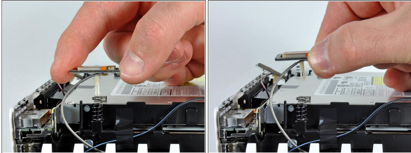
*(i)* The two Bluetooth antenna boards simply lift off the internal frame.
