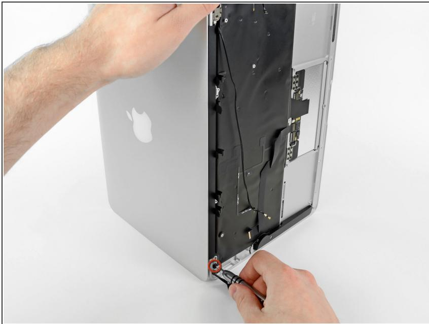
ⓘ Open the display until it is perpendicular to the upper case and place it on a table as shown.
