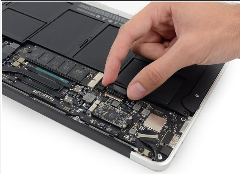
⚠ In this step you will disconnect the battery to help avoid shorting out any components during service.
