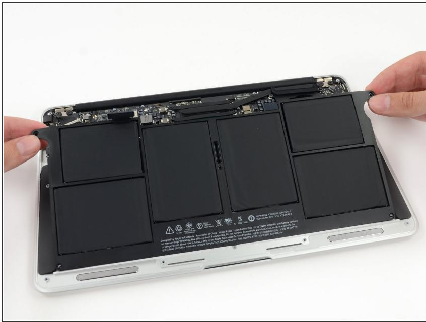
**⚠** When handling the battery, avoid squeezing or touching the six exposed lithium polymer cells.
