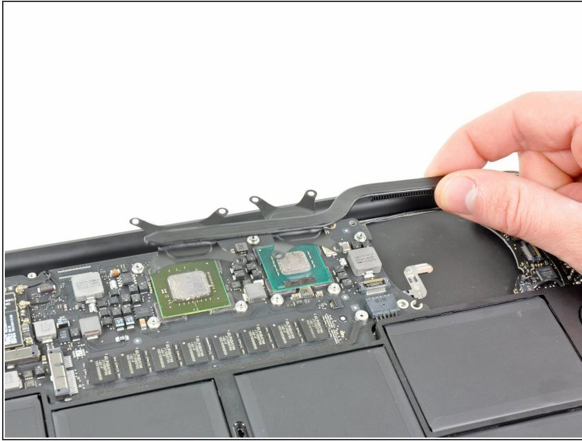
**i** If the heat sink seems to be stuck to the logic board after removing all eight screws, use a spudger to carefully separate the heat sink from the faces of the CPU and GPU.
