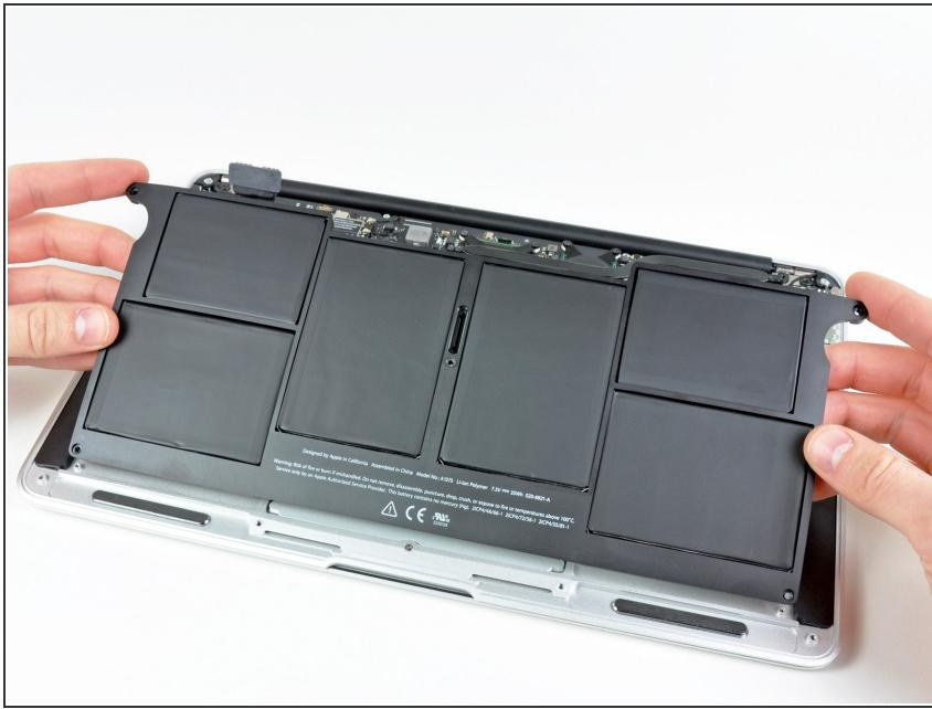
**⚠** Do not touch or squeeze the six lithium polymer cells when handling the battery.
