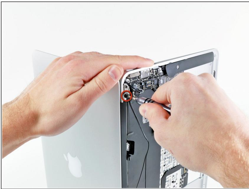
**⚠** Before removing the last display screw, be sure to hold the display and upper case steady with your other hand. Failure to do so may allow the components to fall onto the table, causing potentially expensive damage.
