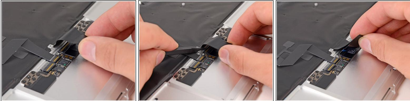
*(i)* The ZIF connector for the keyboard ribbon cable is hidden under the cable itself.
