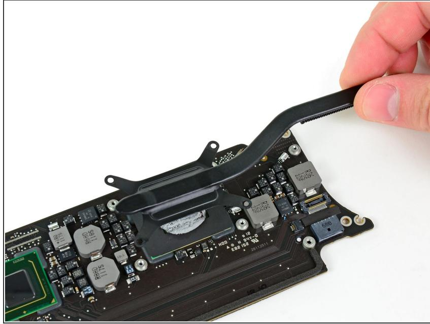
**i** If the heat sink seems to be stuck to the logic board after removing all four screws, use a spudger to carefully separate the heat sink from the faces of the CPU and GPU.
