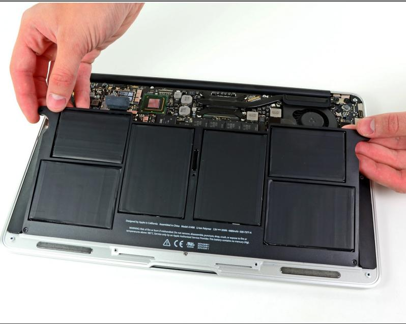
**⚠** When handling the battery, avoid squeezing or touching the six exposed lithium polymer cells.
