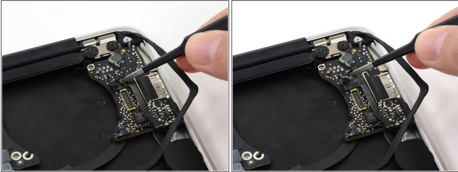
*(i)* If necessary, use tweezers to remove any tape covering the microphone cable ZIF connector.
