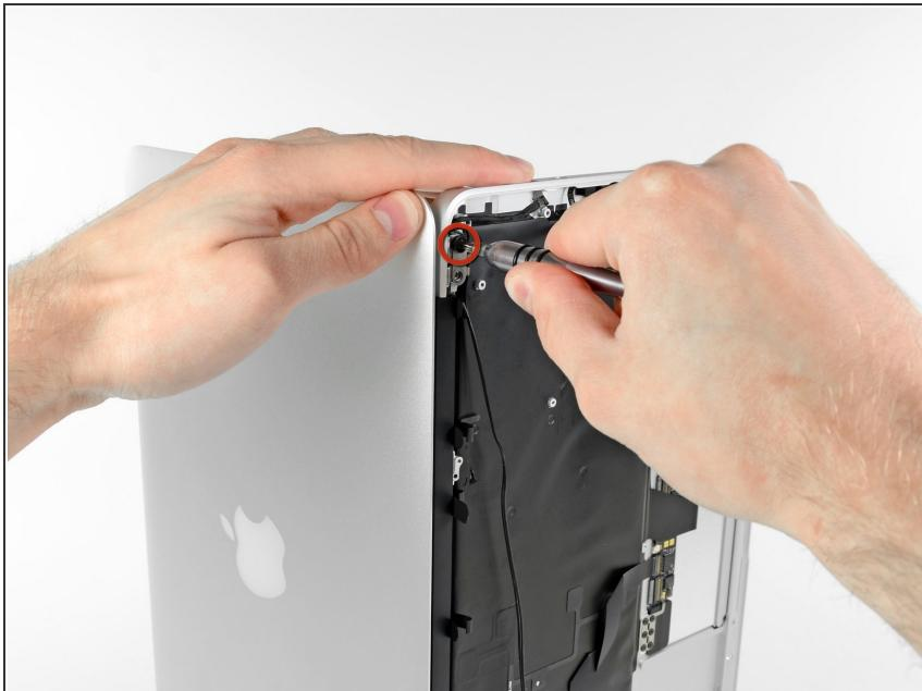
**!** Before removing the last display screw, be sure to hold the display and upper case steady with your other hand. Failure to do so may allow the components to fall onto the table, causing potentially expensive damage.
