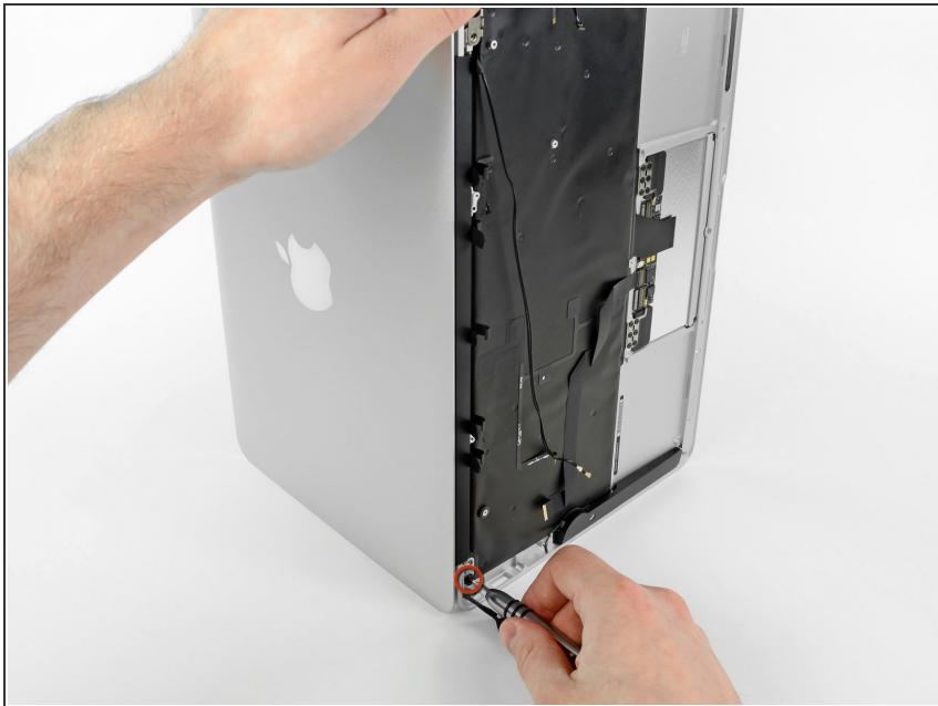
**i** Open the display until it is perpendicular to the upper case and place it on a table as shown.
