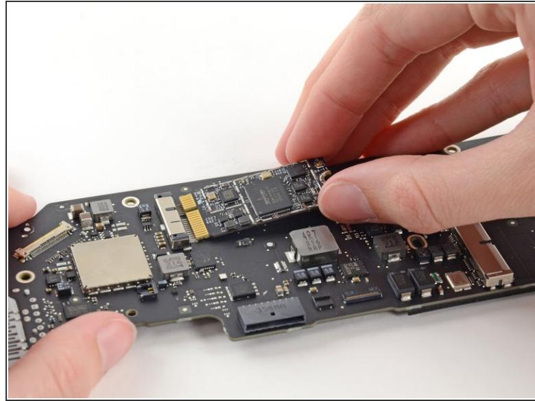
! To avoid damaging its socket, do not lift the end of the AirPort/Bluetooth board excessively.
