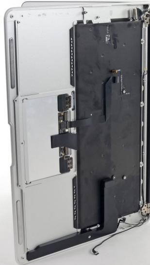
*(i)* Open the display so that it is perpendicular to the upper case and place it on a table as shown.
