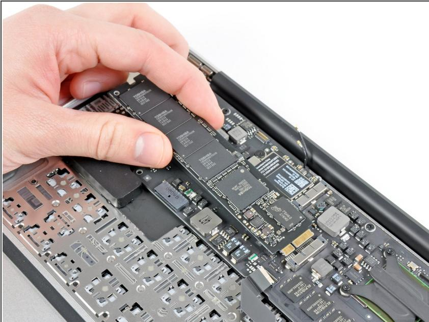
⚠ Do not lift the end of the SSD excessively.
