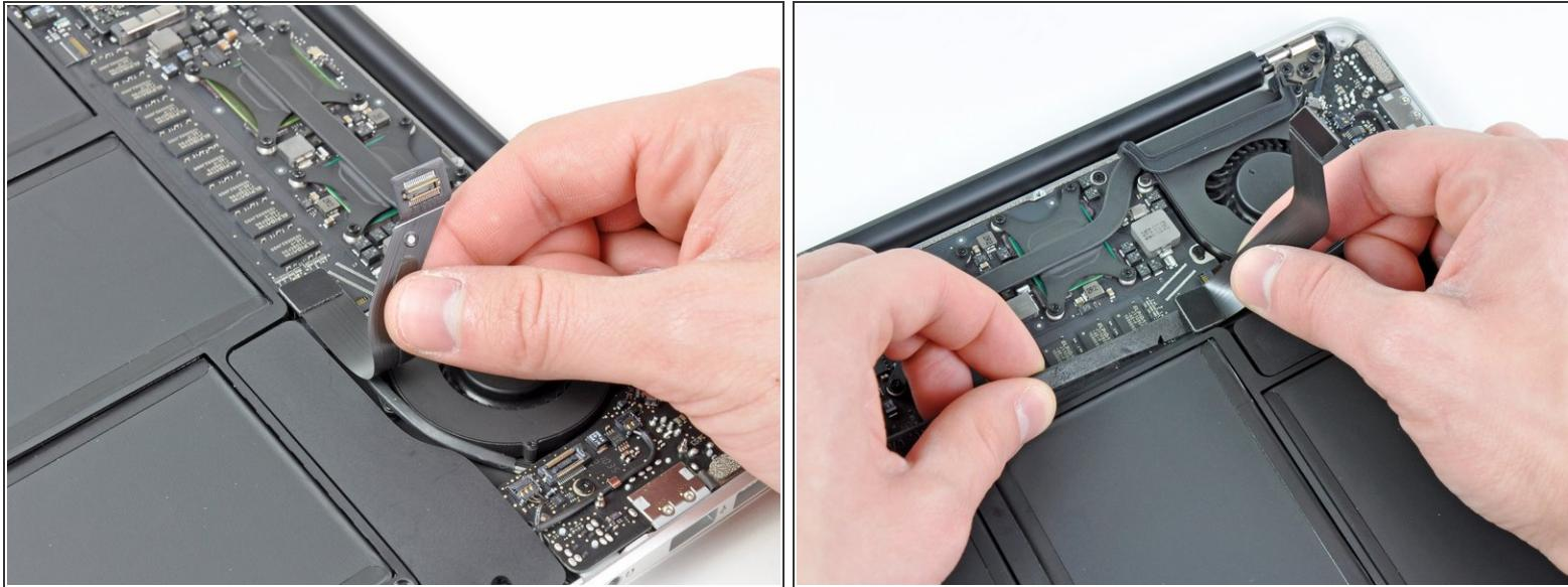
⚠ The following connector has an especially deep socket. Use care when disconnecting it.
