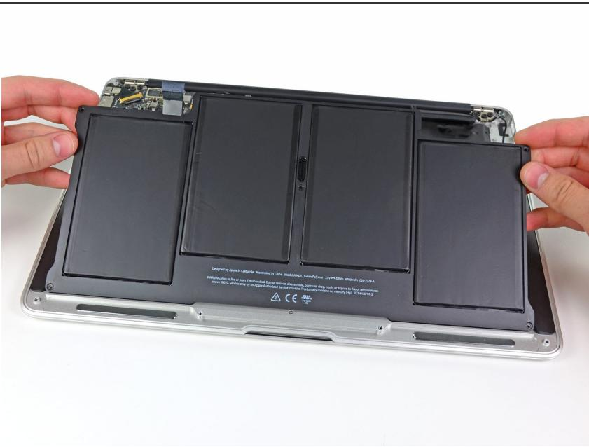
**⚠** When handling the battery, avoid squeezing or touching the four exposed lithium polymer cells.
