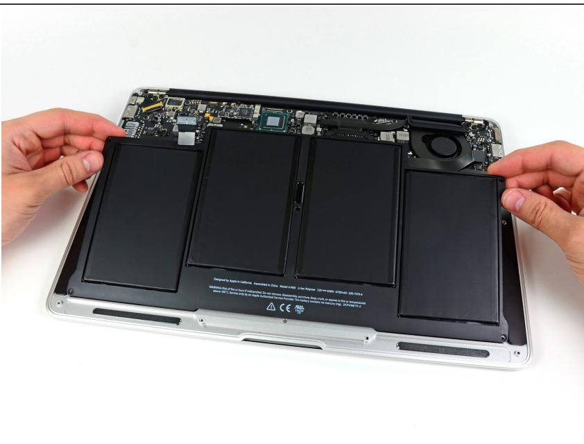
**⚠** When handling the battery, avoid squeezing or touching the four exposed lithium polymer cells.
