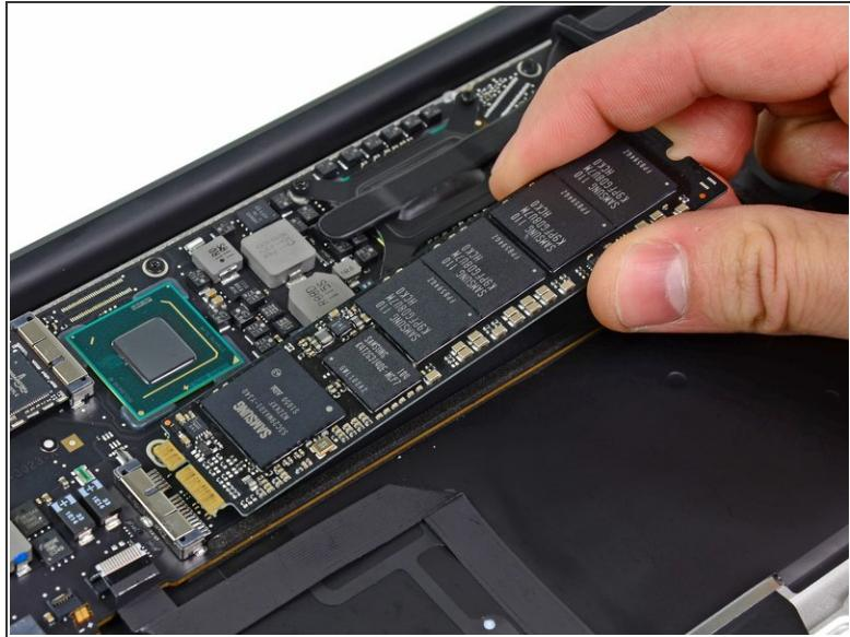
⚠ To avoid damaging its socket, do not lift the end of the SSD excessively.
