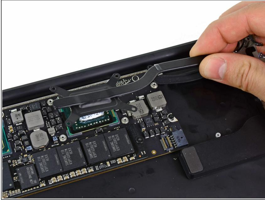
**i** If the heat sink seems to be stuck to the logic board after removing all five screws, use a spudger to carefully separate the heat sink from the faces of the CPU and GPU.
