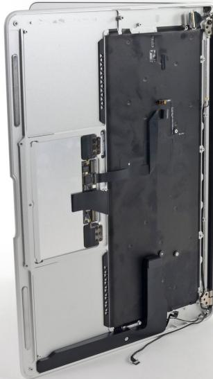
*(i)* Open the display so that it is perpendicular to the upper case and place it on a table as shown.
