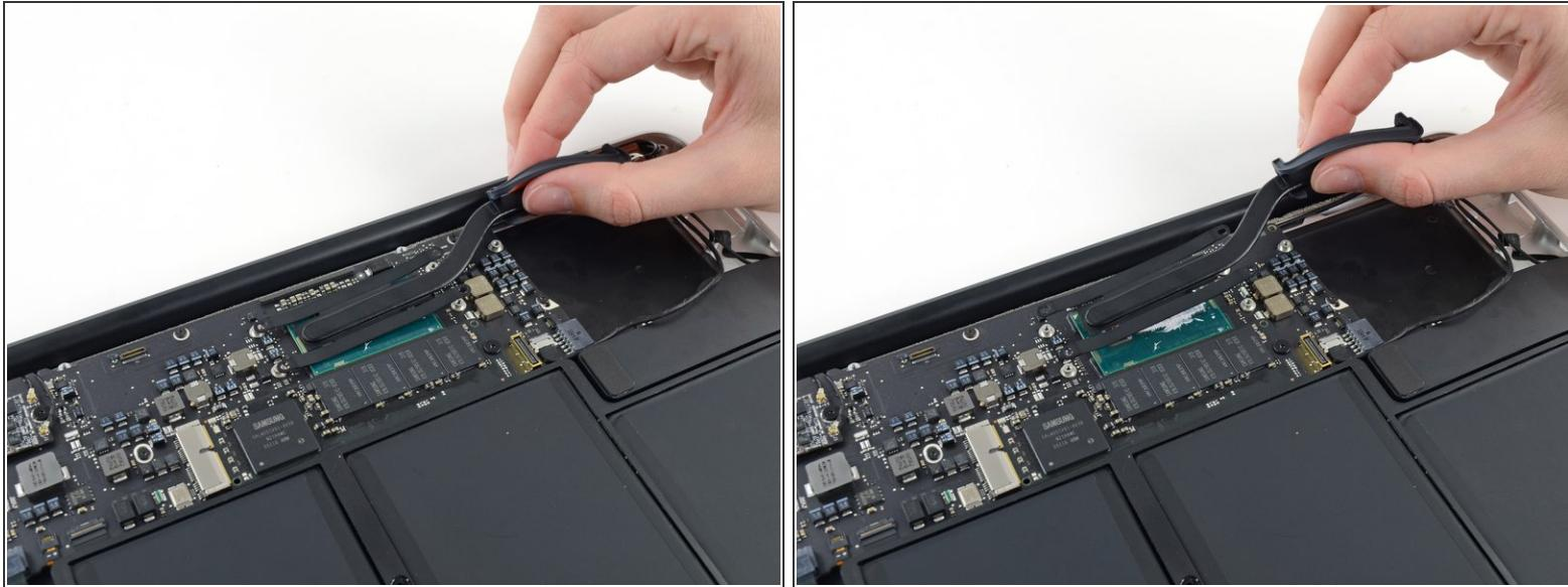
*(i)* If the heat sink seems to be stuck to the logic board after removing all five screws, use a spudger to carefully separate the heat sink from the faces of the CPU and GPU.
