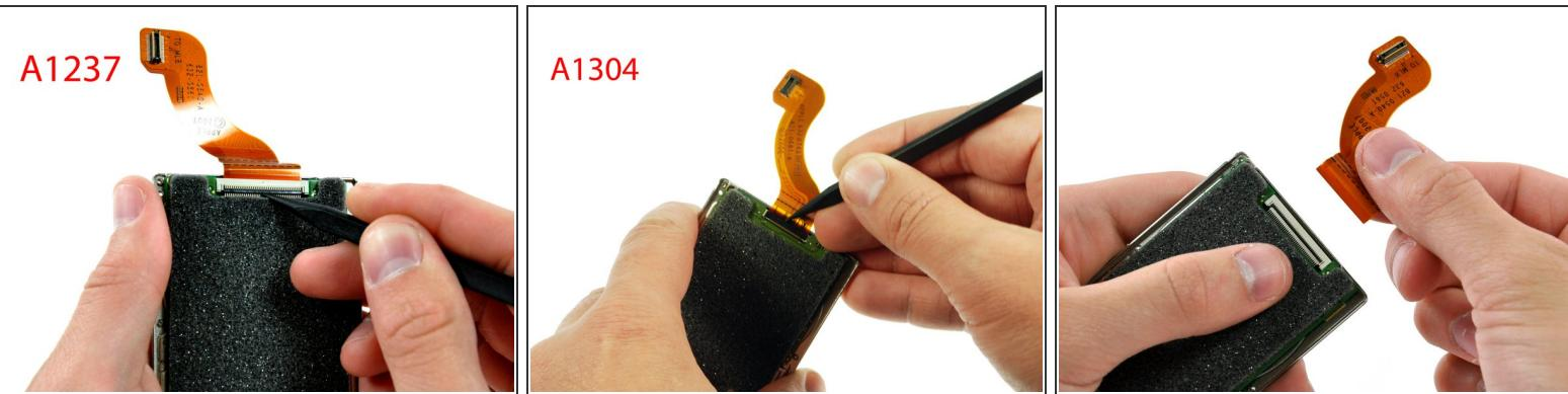
**⚠** The two different versions of MacBook Air have different hard drive connectors. Failure to perform the action appropriate to your machine will damage your hard drive! Be very careful when disconnecting the hard drive cable. The ZIF connectors are fragile.
