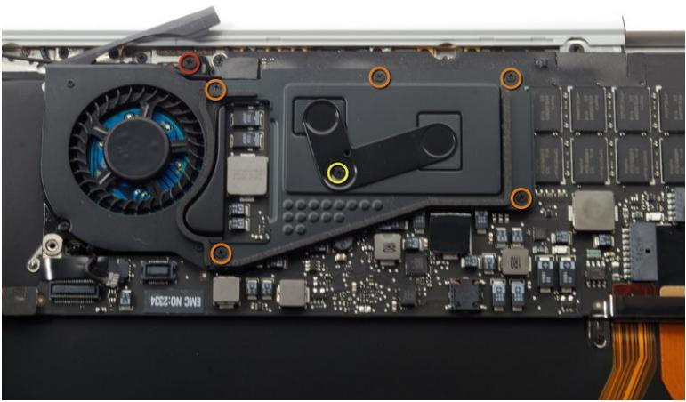
ⓘ If you have the original version of the MacBook Air (A1237), refer to picture 1. Remove the following screws securing the heat sink to the logic board:
