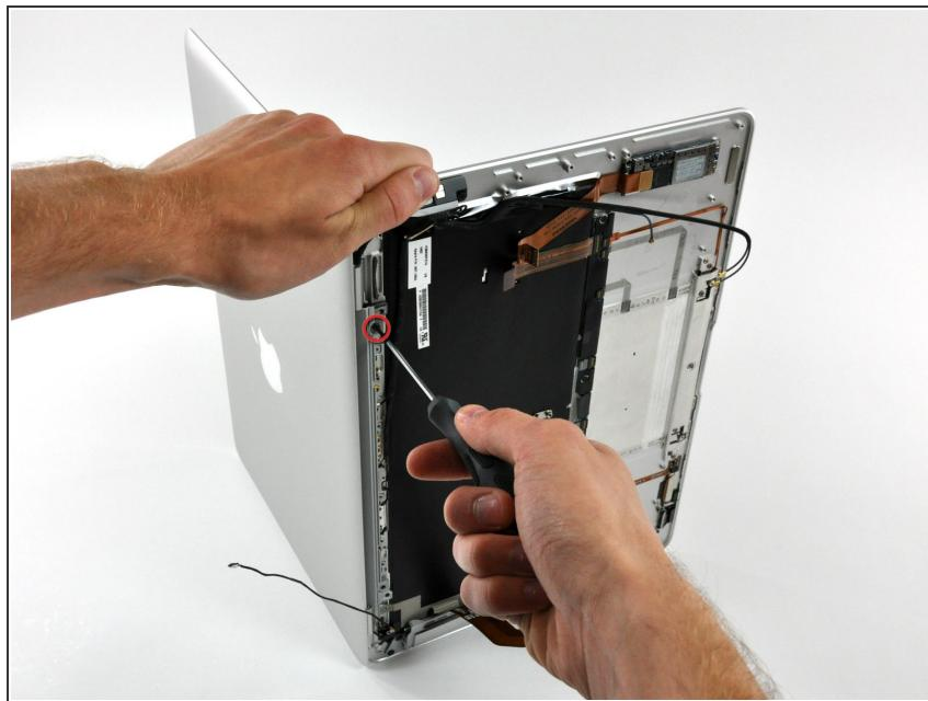
**i** Be sure to hold the Air together while you remove the last Torx screw. Failure to do so may cause the display/upper case to fall, potentially damaging both components.
