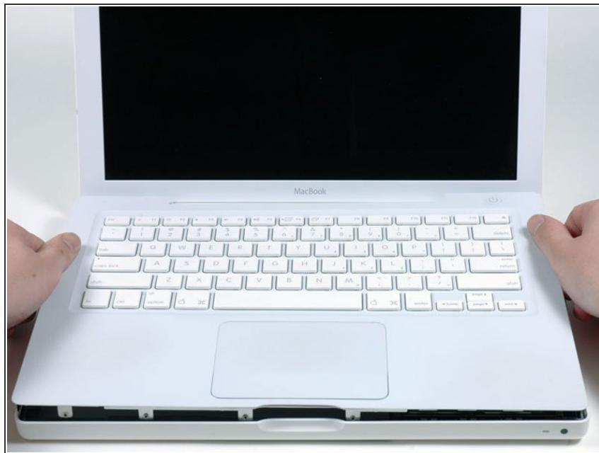
**⚠** There's a trackpad and keyboard ribbon connecting the upper case to the logic board, so don't pull the upper case off entirely just yet.
