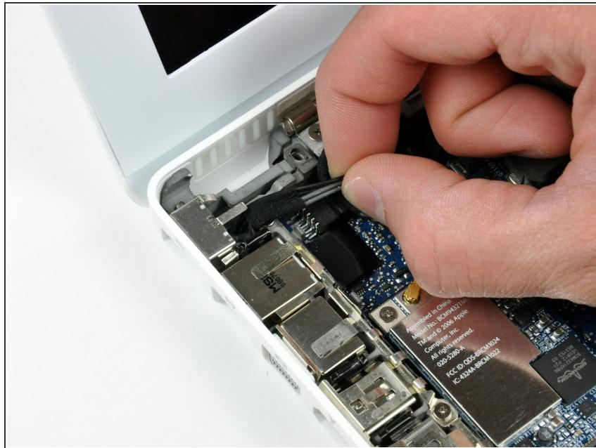
**i** The MagSafe board connector is underneath the wires, be sure to pull on the connector itself pulling parallel to the socket.
