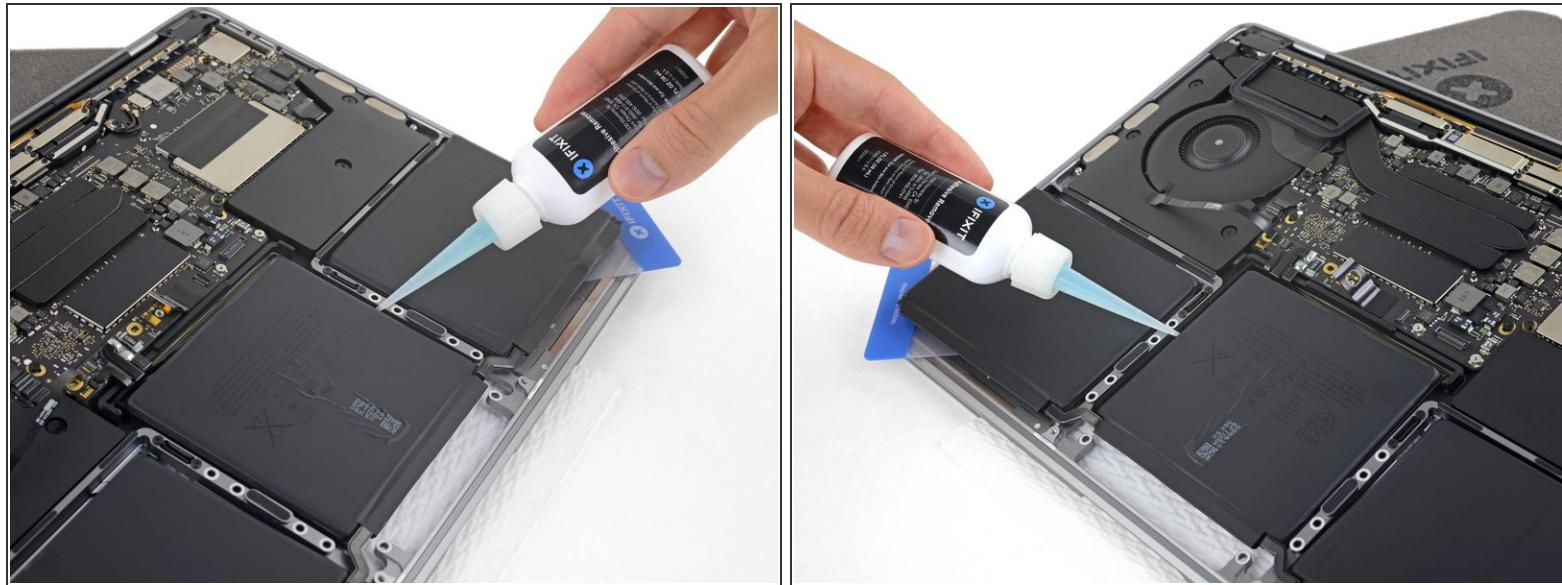
*(i)* [Cutouts in the aluminum case](#) between the center battery cell and trackpad may prevent the adhesive remover from flowing all the way underneath the battery.
