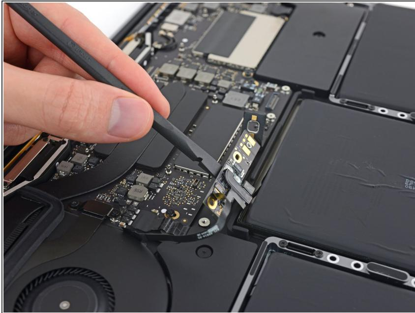
**i** The battery board is permanently attached to the battery. Check to make sure it has adequate clearance to come out together with the battery, without snagging on other components.
