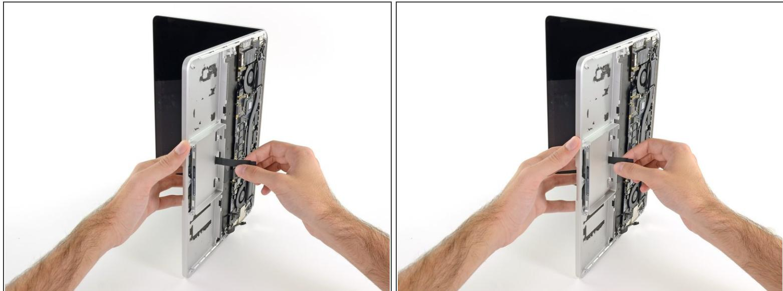
*(i)* To avoid scratching the display, open the computer about 90° and set it on end.
