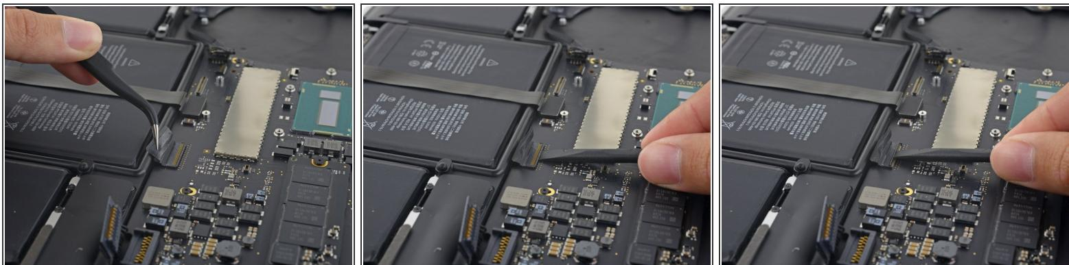
*(i)* If necessary, peel back any tape covering the keyboard cable connector.
