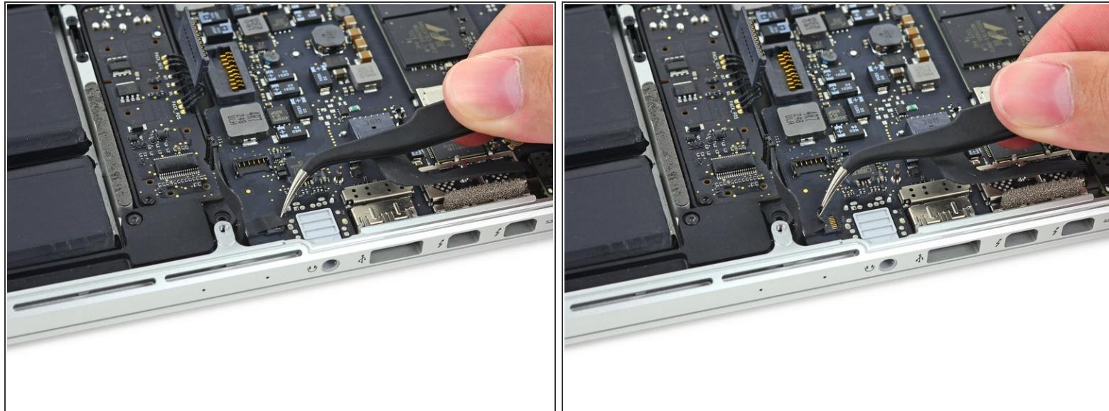
ⓘ If necessary, peel back any tape covering the microphone cable ZIF connector.
