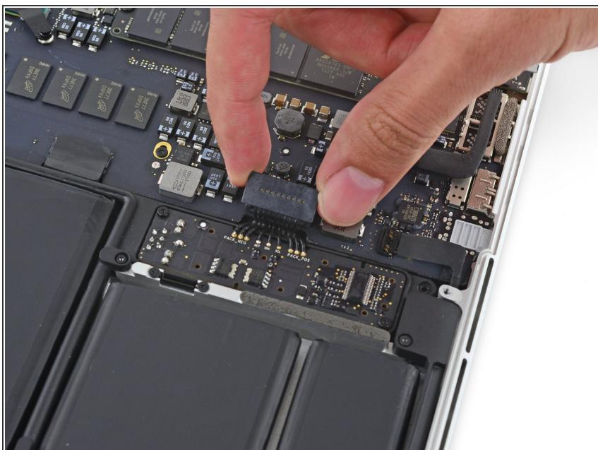
➡ Bend the battery connector up out of the way to prevent accidental contact with its socket during your repair.
