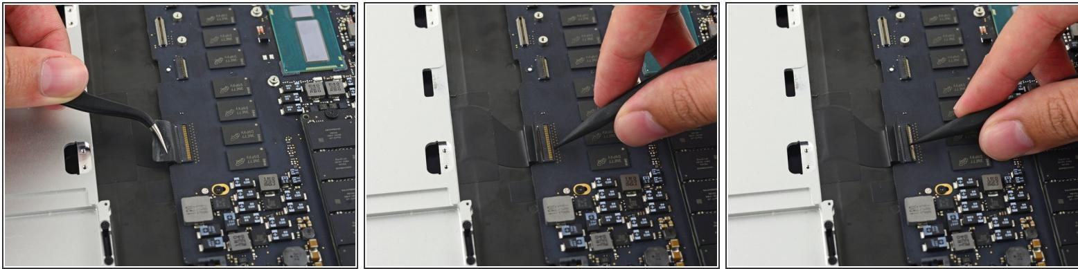
ⓘ If necessary, peel back any tape covering the keyboard cable connector.
