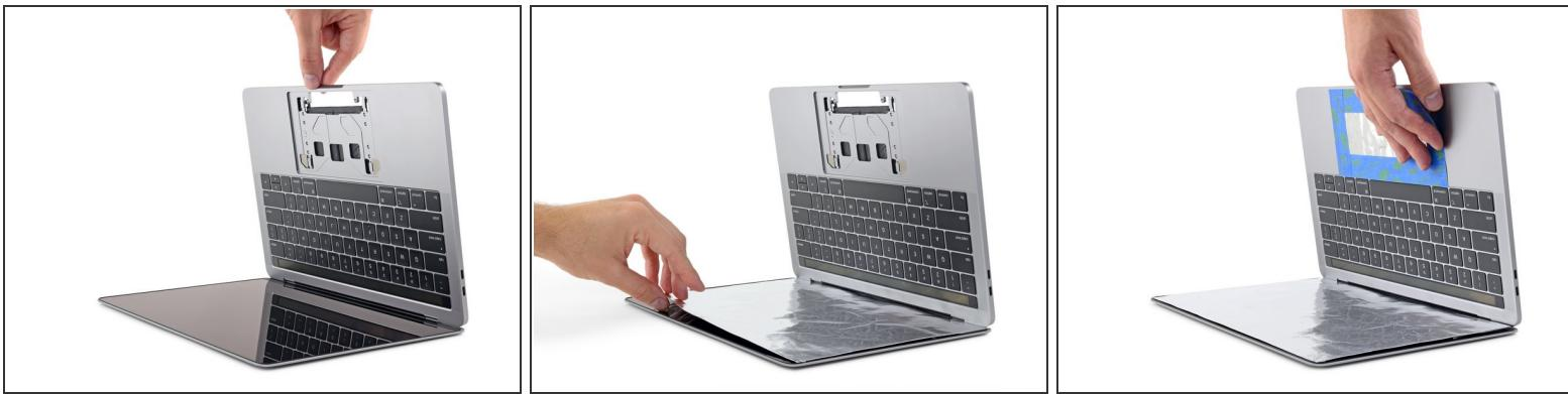
**⚠** The liquid adhesive remover provided in your kit can cause damage if it contacts the MacBook Pro's display or keyboard.
