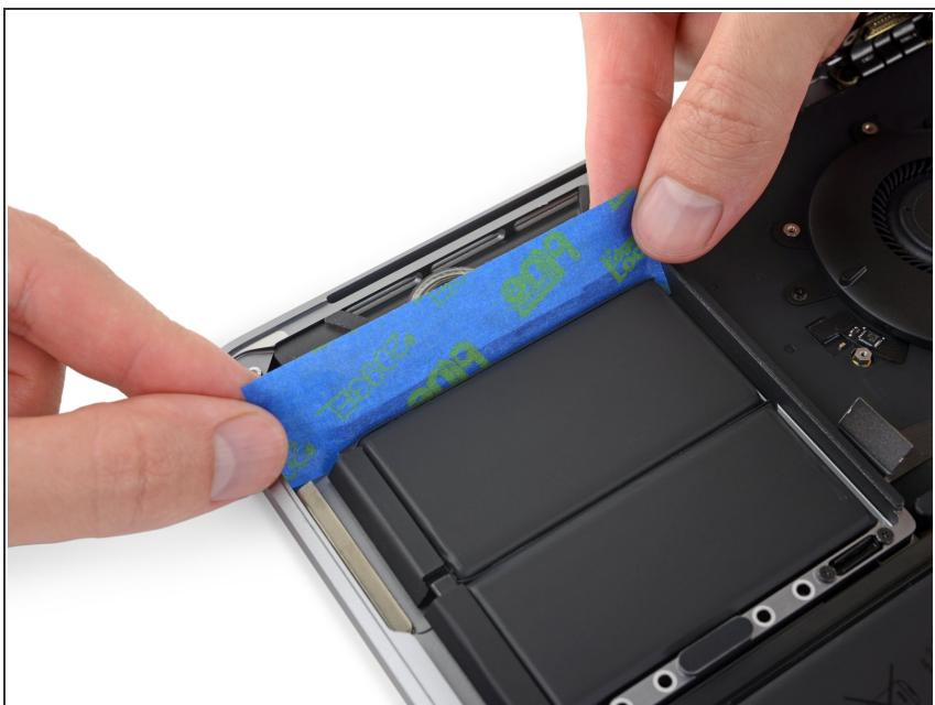
**i** Before removing the battery, it's important to protect the speakers on either side. The speakers are glued down just like the battery—so if the liquid adhesive remover gets under the speakers, they may come loose and rattle after your repair.
