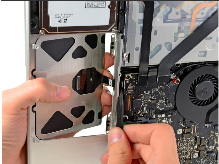
**i** If you are installing a replacement trackpad that didn't come with the attached flex cable, you'll need to use the cable from your old trackpad.
