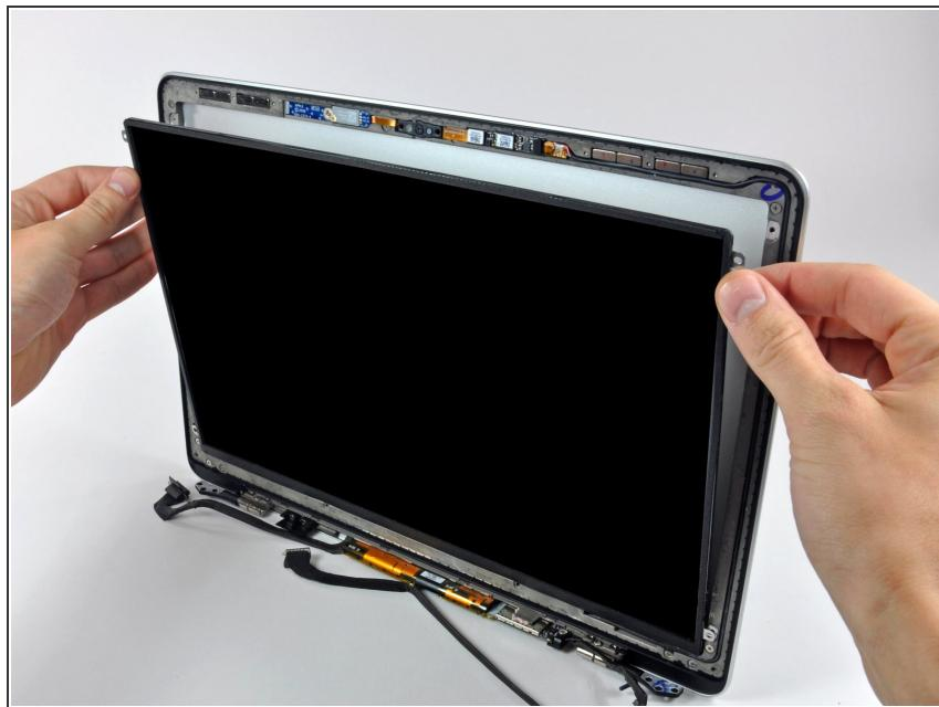
**⚠** Do not try to remove the LCD yet. The circuitry along its lower edge is wedged in a gap along the lower edge of the display recess in the aluminum display assembly.
