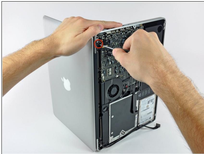
⚠ Be sure to hold the display and upper case together with your left hand. Failure to do so may cause the freed display/upper case to fall, potentially damaging each component.
