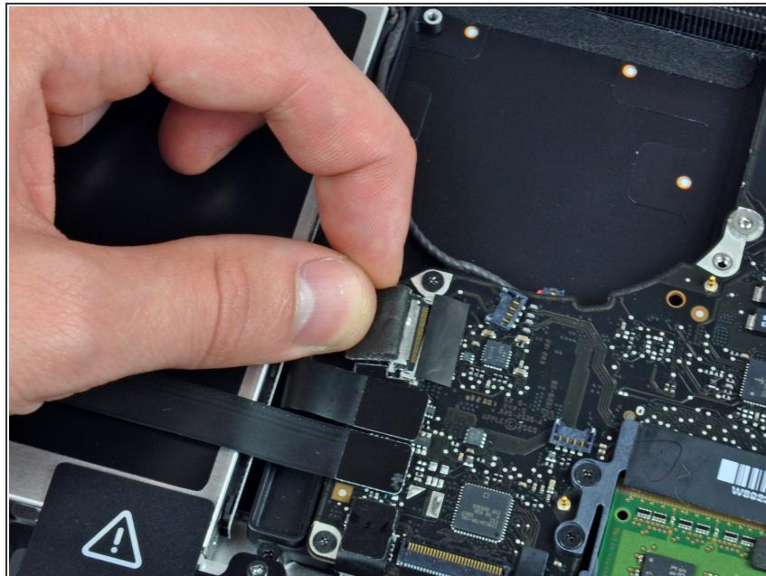
⚠ In this step you will disconnect the camera cable. Most machines will have a small self adhesive plastic retainer stuck to the logic board to keep the connector in place. Before disconnecting the cable, be sure this retainer is moved out of the way.
