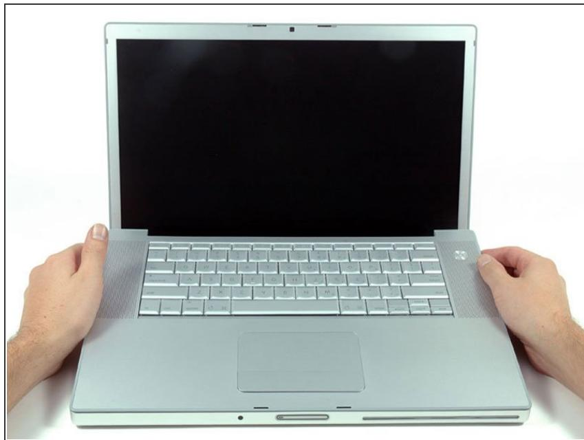
**i** Do not yank the upper case off quickly. The case is attached to the logic board via a ribbon cable.
