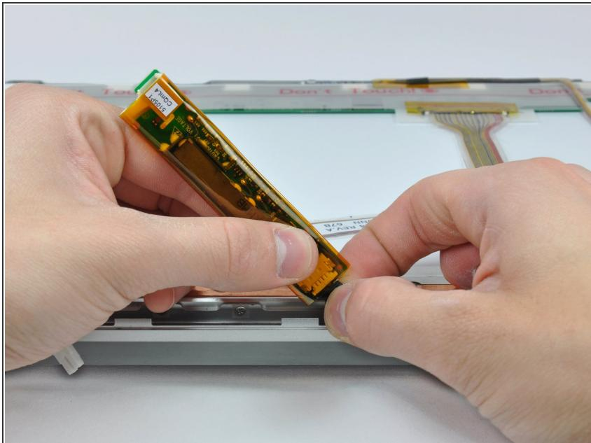
! Be cautious to not put any strain on the inverter cable ground loop, as it is a very thin and delicate wire.
