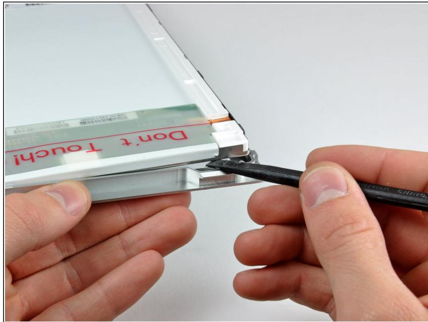
**i** The next few steps will require you to separate the LCD from the adhesive applied to the upper and lower edges of the front bezel. A heat gun may be helpful to soften the adhesive to prevent damaging the LCD panel during removal.
