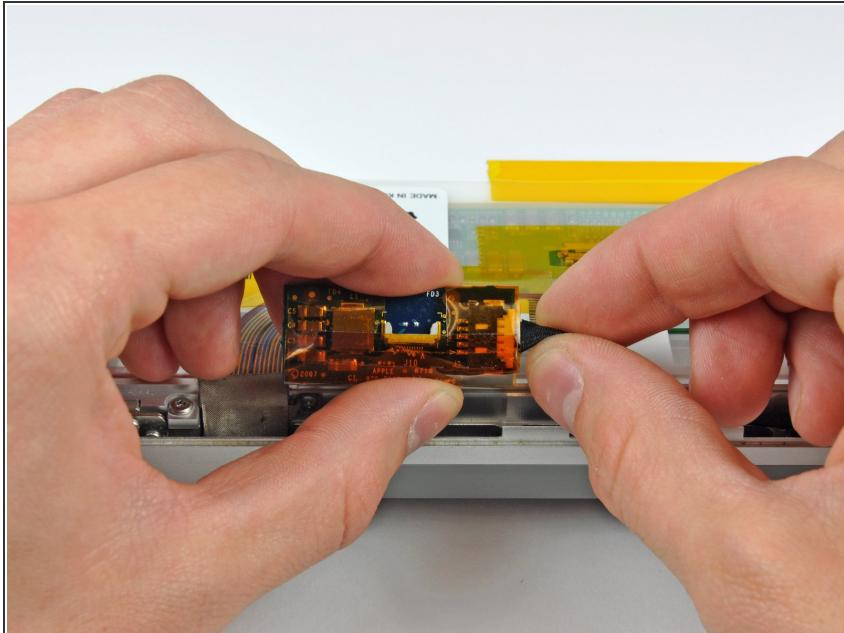
! Do not put any excessive strain on the LED driver cable ground loop. It is a very thin and delicate wire that is easily broken.
