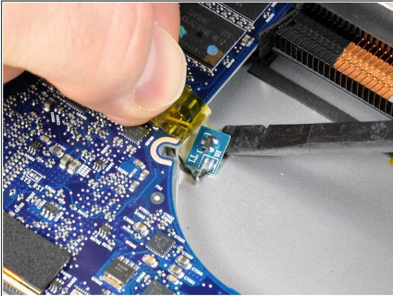
**⚠** Use caution when removing the thermal sensor connector. The connector can easily break off the logic board if this step is performed improperly.
