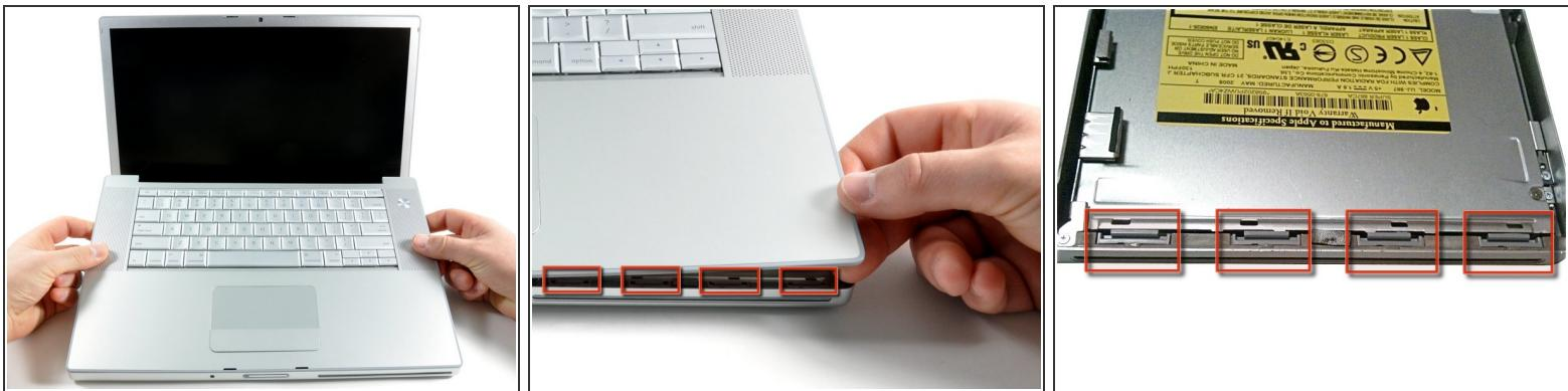
ⓘ Do not yank the upper case off quickly. The case is attached to the logic board via a ribbon cable.
